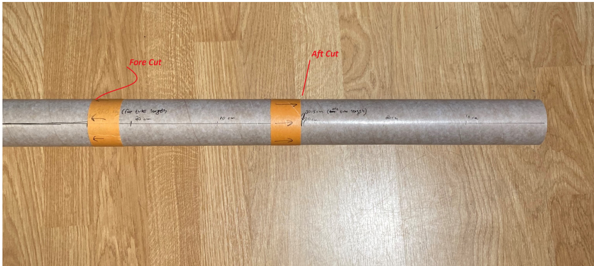
Figure 3: The body tube with segment lengths marked. Fore segment is on the left, aft segment on the right
