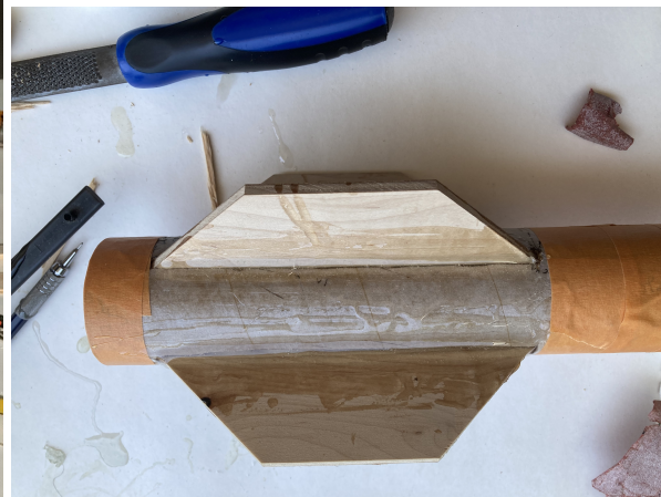
(b) Two fin fillets curing.
