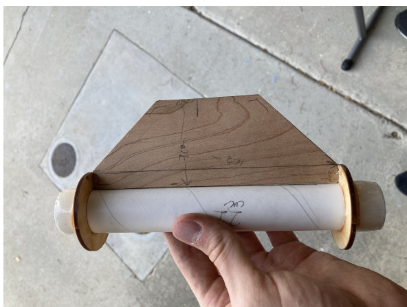
(a) One fin test fit into the motor mount
