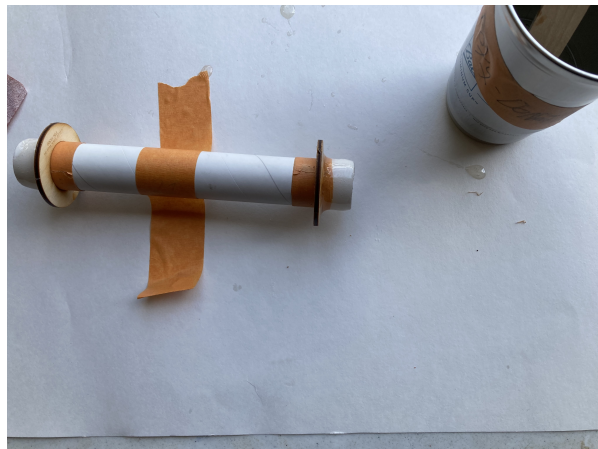
(b) The motor mount curing. Note the removed masking tape under the epoxy fillets.
